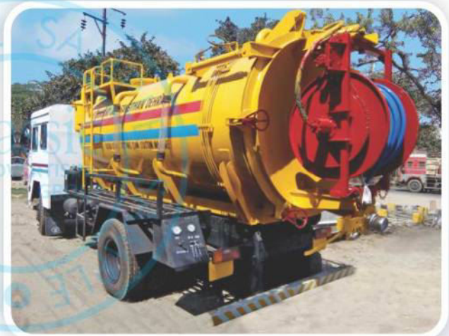
Sewer Jetting cum Suction Machine of 10000 Ltrs.
