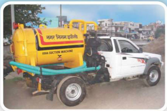
Sewer Suction Machine with Auxiliary Engine
