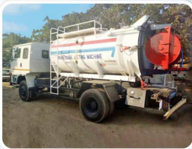
Sewer Jetting cum Suction Machine of 8000 Ltrs.
