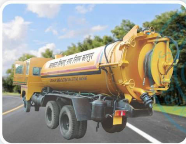
Sewer Jetting cum Suction Machine 12000 Ltrs.
