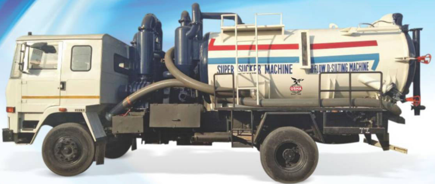
Hi-Power Suction Machine with Blower (8000 Ltrs. Capacity)
