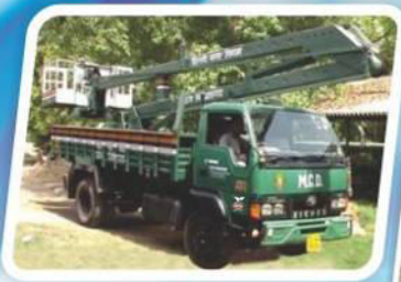
15 Mtrs. Sky Lift with Slew Bucket
