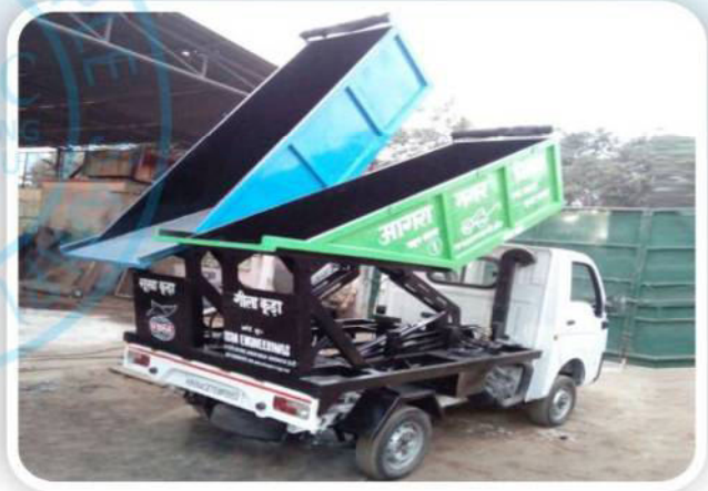
Twin Bin Hopper with Individual Hydraulic System
