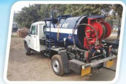
Sewer Jetting Machine of 1500 Ltrs. on Mahindra Bolero Pick up
