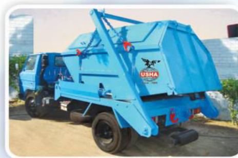
Single Bin Dumper Placer with Container
