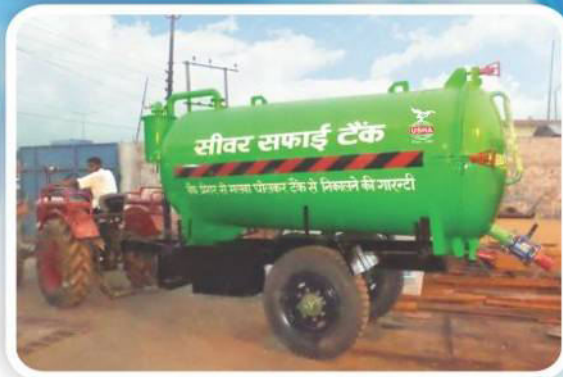
Tractor coupled Suction Machine
