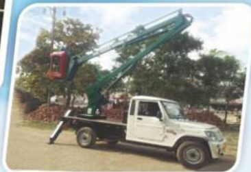
2 Boom type Sky Lift of 9 Mtrs. on Mahindra Bolero
