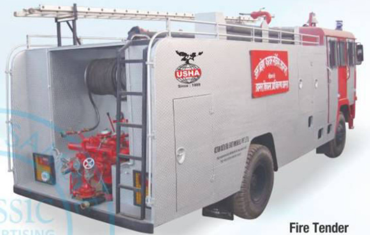
Water Tanker with Pumps
