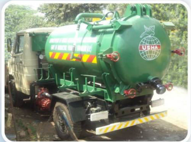
Sewer Suction Machine of 3000 Ltrs.
