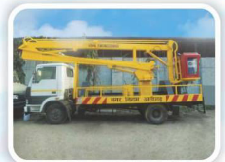
3 Boom Type Hydraulic Platform 15 Mtrs.
